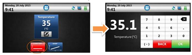
Depress the icon to activate the numeric keyboard, and enter a temperature value between -5 and 65°C. Confirm by "OK".
